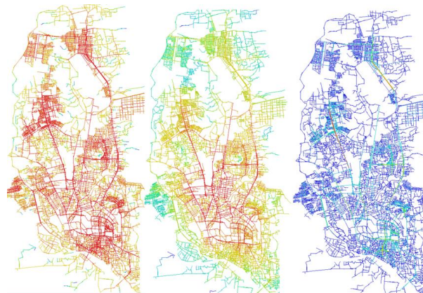
Figure 4: Axial Map of Dhaka City with Local Integration ( R=40 ) (Left), Global Integration ( R=N ) (Middle), Connectivity (Right)
